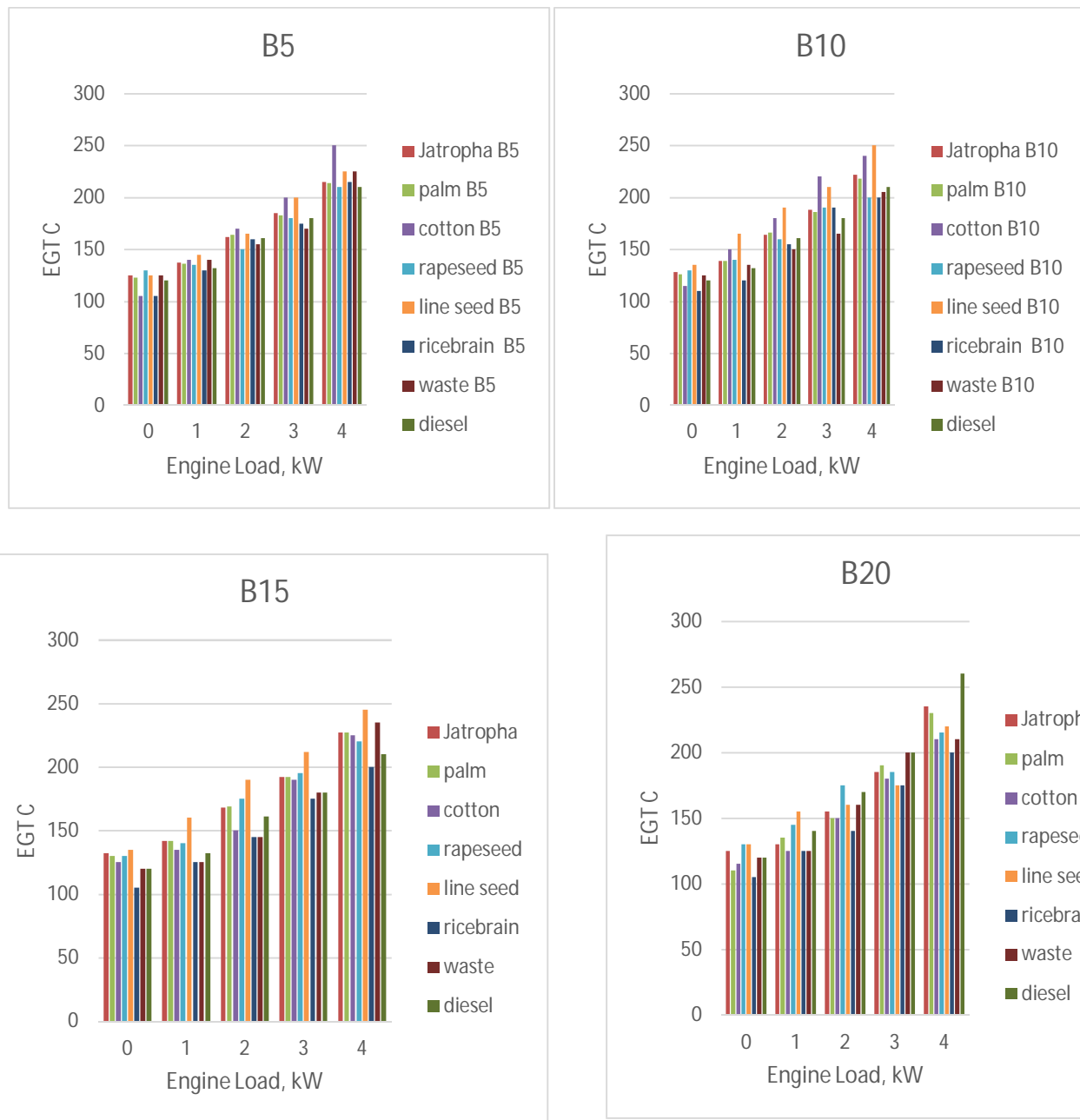
Fig.4. Variation of exhaust gas temperature versus engine load for different fuels.
