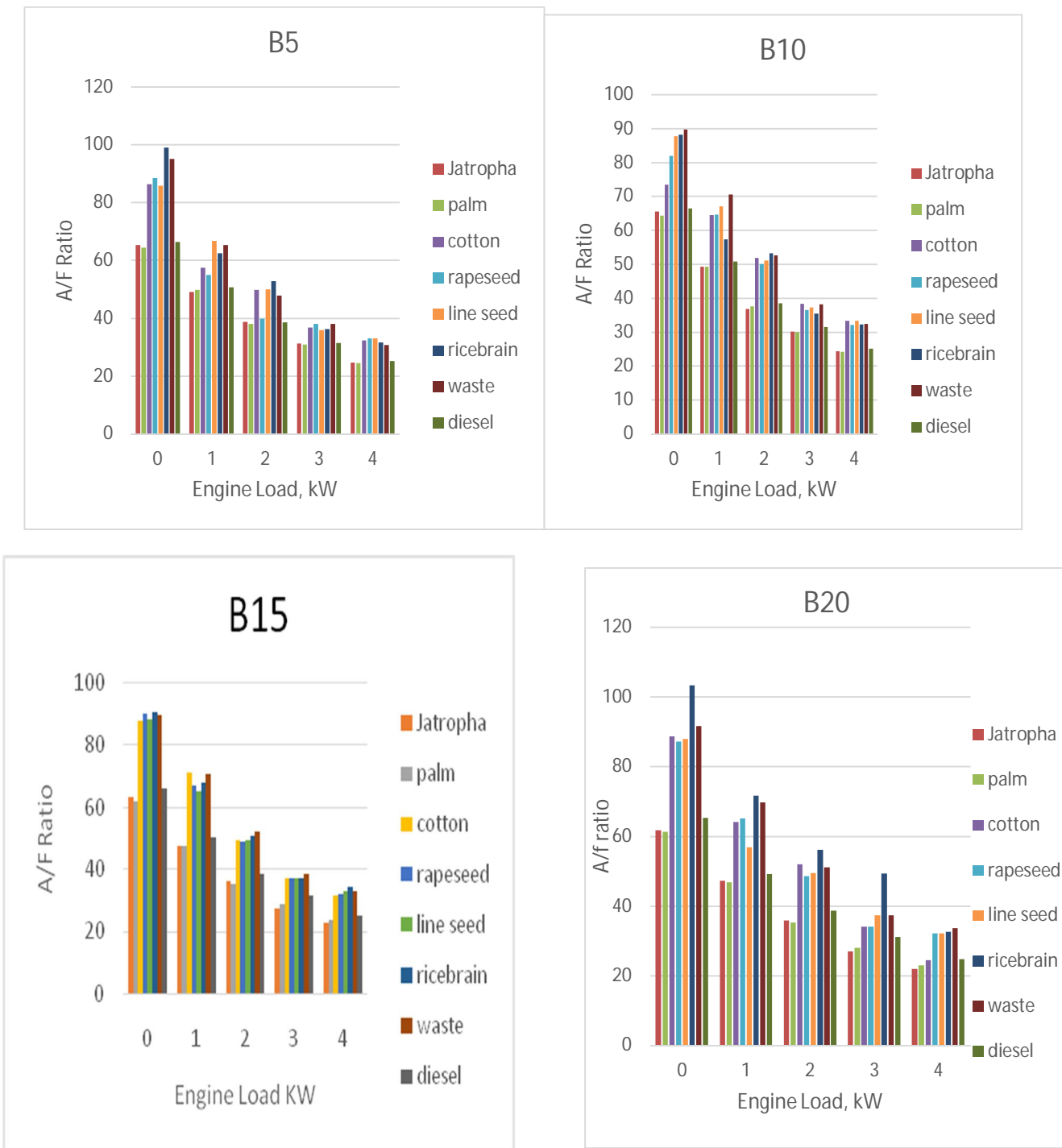
Fig.5. Variation of Air-Fuel ratio with engine load for different fuels.
