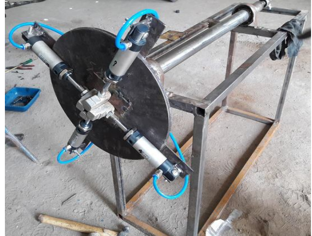
Fig. 3.b. Front View of Pneumatic Chuck
