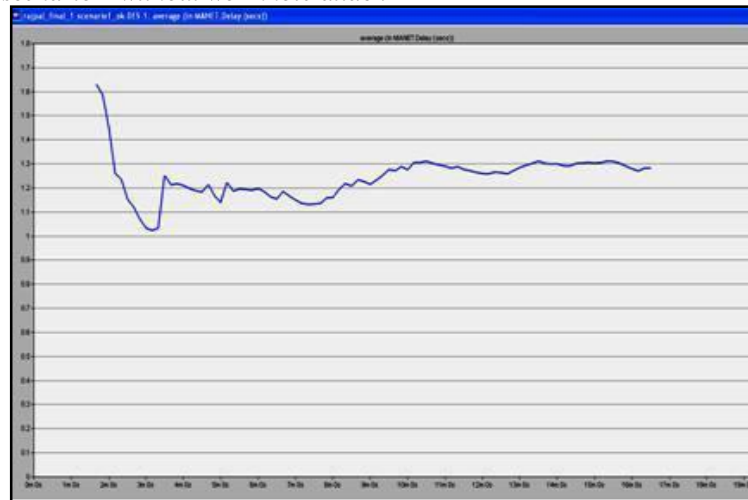
Figure 5.5 Average delays per route in scenario 1 without wormhole attack
