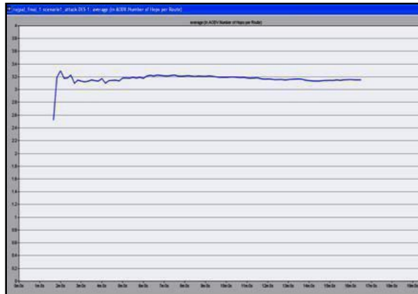
Figure 5.7 Average Hop count per route in scenario 2 with wormhole attack
