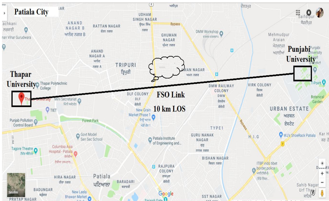
Fig.2 Architecture of FSO link with 10 km Line of sight (Los) [12].
