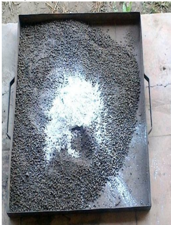
(a) Kuttanad Clay mixed with Lime
