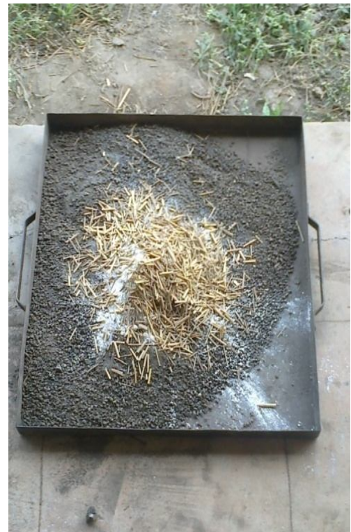
(b) Kuttanad Clay mixed with Lime and Rice Straw
