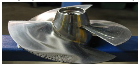
Fig. 1: Cavitation on turbine blade.
