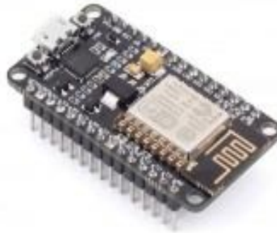
Figure 11: IOT Module with ESP8266
