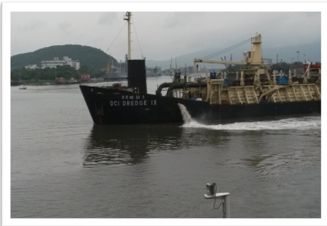
Figure 4.8 Trailer Suction Hopper Dredger dredging at IHC area
