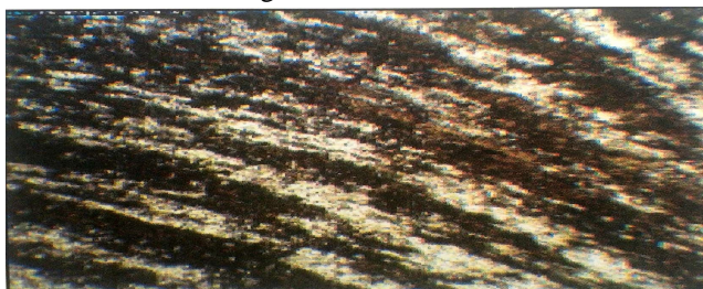
Fig.7: Microstructural view of AA 2014T6 FSW joint
