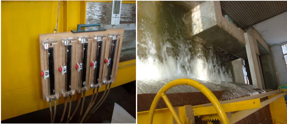
Fig.2(a-d):Starting with clockwise from top left): (a)&(b)Side & top view of Series of pitot static tubes fitted to stand with transparent pipes & pointer gauge, (c)D/S tail gate and volumetric tank . (d) Set of Piezometers fitted to wooden board to record pressure with spirit level, digital clock etc.
