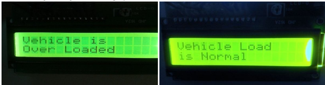
Fig15: Informs the traveler vehicle is overloaded Fig16: Informs the traveler that vehicle load is normal
