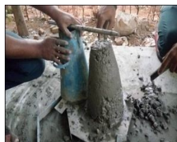
Fig: 1 Slump cone test
