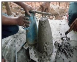
Fig: 1 Slump cone test
