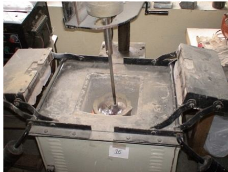
Stir casting Process
