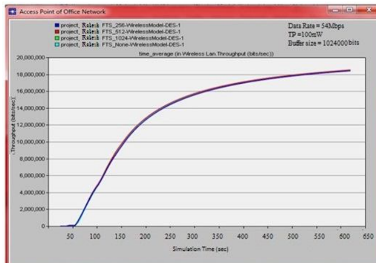
Fig. 6 Throughput results for different fragmentation threshold
