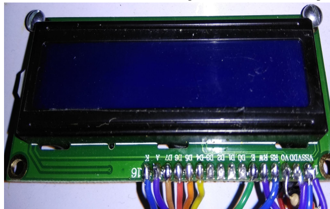
Fig 5 a) Interfacing of LCD with Arduino pins
