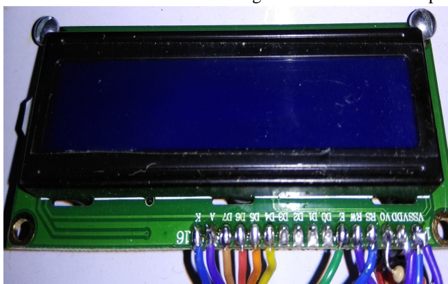
Fig 5 a) Interfacing of LCD with Arduino pins
