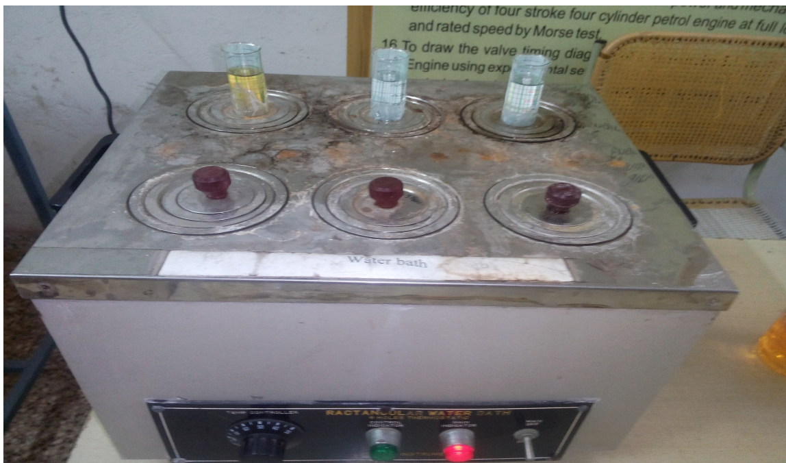
Fig : Experimental setup for measurement of diffusivity.
