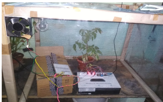
Figure 4(b): Photograph of Polyhouse Prototype
