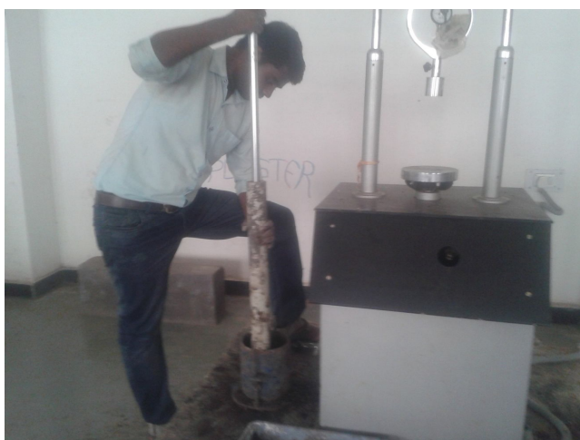
Figure 3: Heavy Compaction Test
