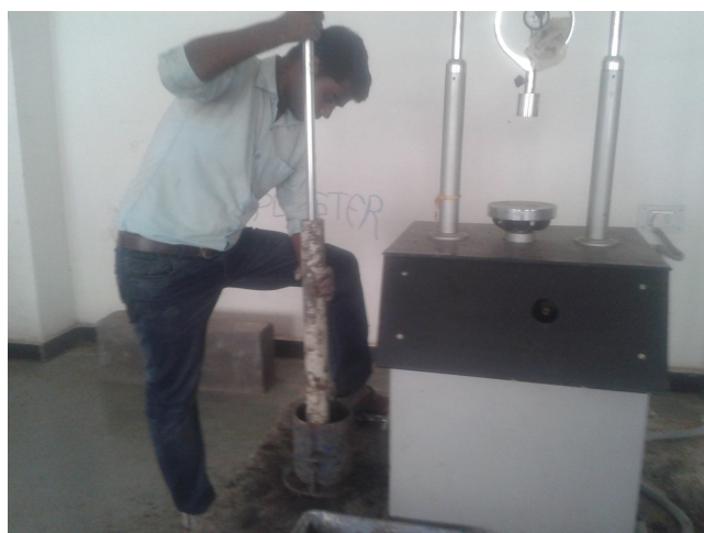
Figure 3: Heavy Compaction Test
