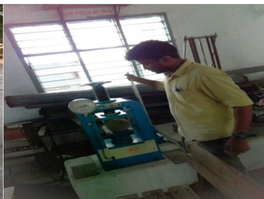
Testing of Cubes
