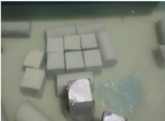
Curing of cubes
