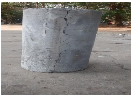
Failure of Cylinder
