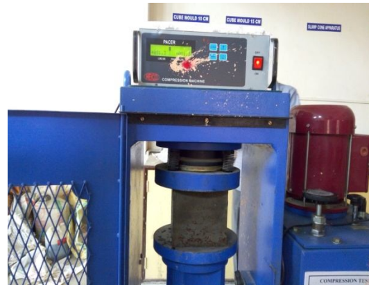
Testing of Cubes
