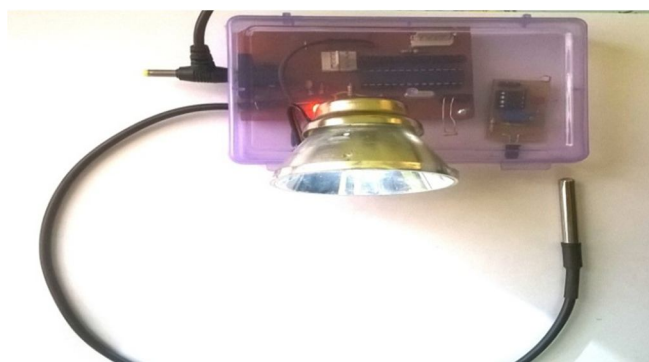
Fig 3 Li-Fi based implemented Wireless Sensor Node
