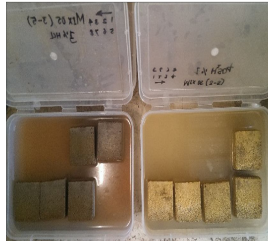
Fig. 4 Acid boxes with mortar
