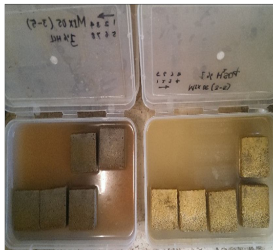
Fig. 4 Acid boxes with mortar
