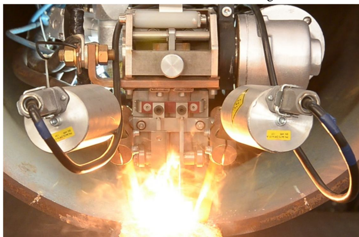
Figure # 3 Resistance Electro slag Strip Cladding inside Pipe
