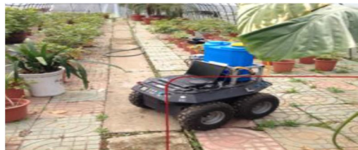
Fig. 3 Greenhouse turning tests of mobile robot
