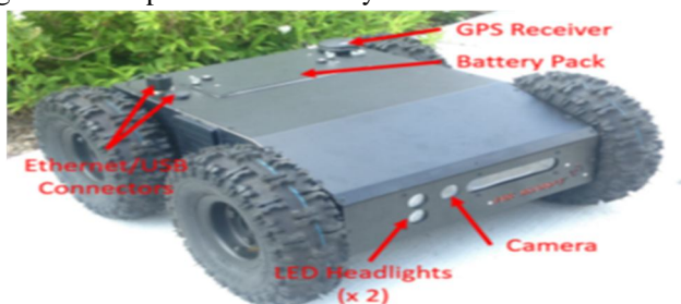
Fig. 1 Jaguar 4x4 platform configuration
