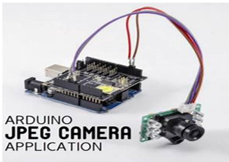
Fig 5: Interfacing Of Arduino With Web Camera
