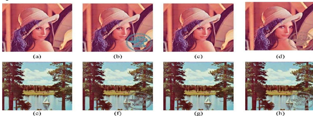
Fig.3. Experimental results of monochrome watermark embedding and removal. (a) Image Lena. (e) Image Sailboat. (b), (f) Watermarked image of (a) & (d), respectively. (c), (g) images losslessly recovered from (b) and (f), respectively, with correct keys. (d), (h) images recovered from (b) and (f) with in correct key
