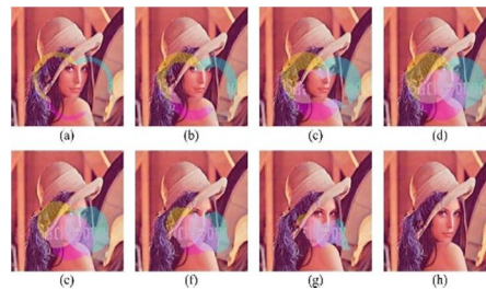
Fig.5. Illustration of pixel processing order in watermark embedding and removal. (a) - (b) intermediate results of image watermarking when 25%, 50%, 75%, and 100% of the watermark pixels have been processed, respectively. (e) - (h) intermediate results of image recovery when 25%, 50%, 75%, and 100% of the watermark pixels have been recovered, respectively.
