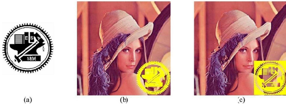
Fig. 2. Illustration of pixels in a watermark. (a) Amonochrome watermark. (b) Area of P (yellow pixels). (c) Area of P 1 (yellow pixels)
