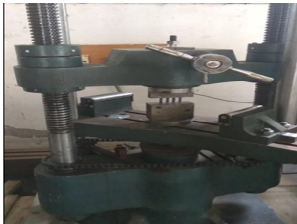
Fig.2.3 Die mounted on UTM machine
