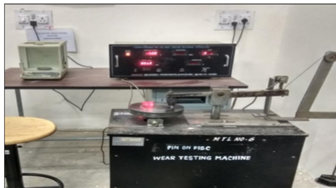
Fig: 2.5 Pin on Disc testing machine
