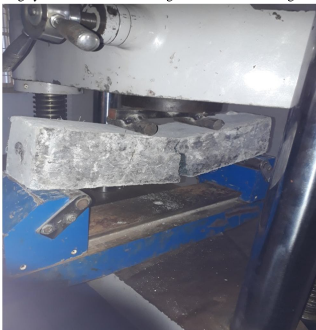
Fig. 12 Flexural strength Test
