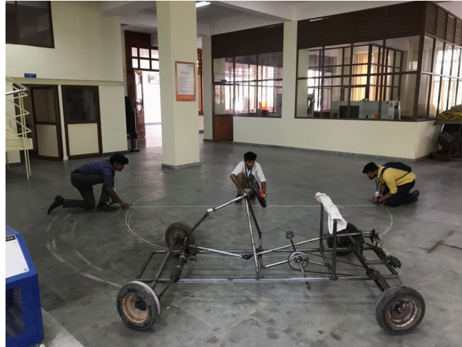
Figure 8.2: Diameter measurement of the traced circle
