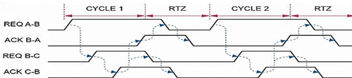
Fig. 6 4-Phase handshaking communication, [4]
