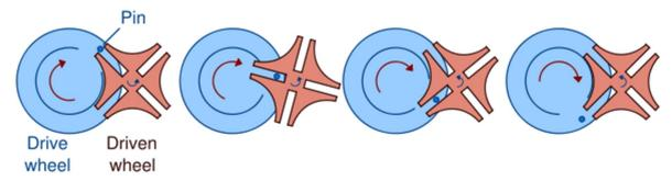
The most common arrangement of Geneva wheel mechanism, The driven wheel has four slots and thus advances the driven by one step at a time (each step being 90 degrees) for each full rotation of the master wheel. The whole system work safely due to proper maintainance and regular lubrication.
