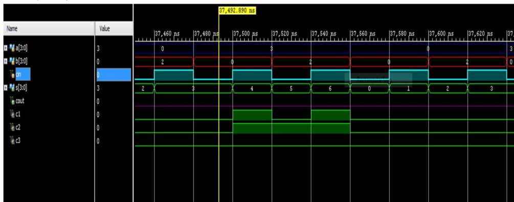
Fig.7 Simulation Results of Ripple Carry Adder
