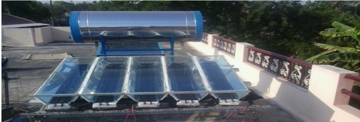
Fig no: 7 Construction of v-trough
