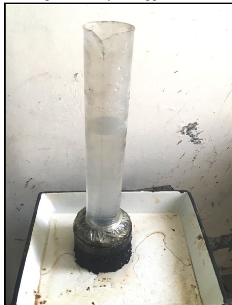
Fig. 5 Permeability test of Bituminous Samples
