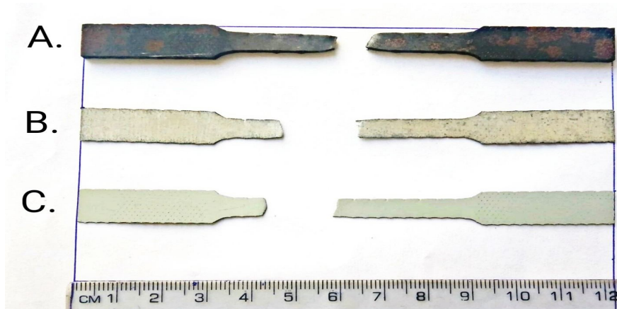
Fig. 3 Tensile specimens after tensile test of different samples i.e.; A. (HR Sample), B. (CR Sample) and C. (Galvanized Steel Sample)
