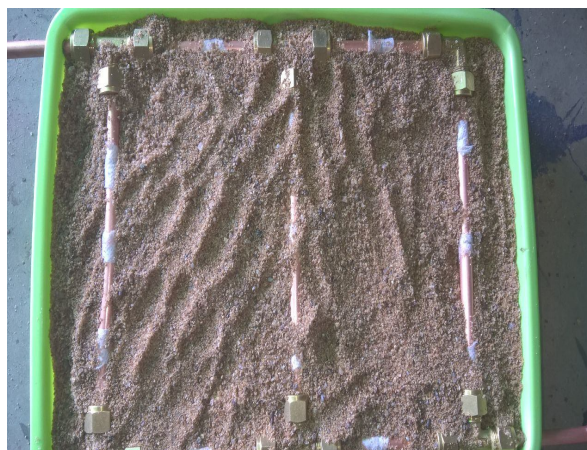
Figure 1: Set-Up of Copper pipes in Sand
