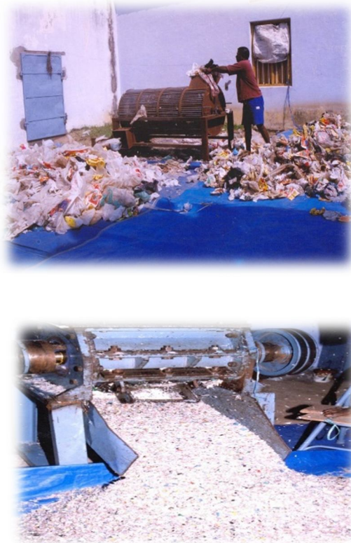
Fig. 2 Shredding of Waste Plastic
