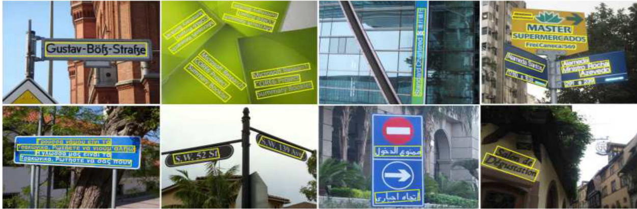
Fig. 3: Text detection examples of the algorithm of Yao et al. [12]. Different from previous methods, which have focused on horizontal or near-horizontal texts, this algorithm is able to detect texts of varying orientations in natural images.
