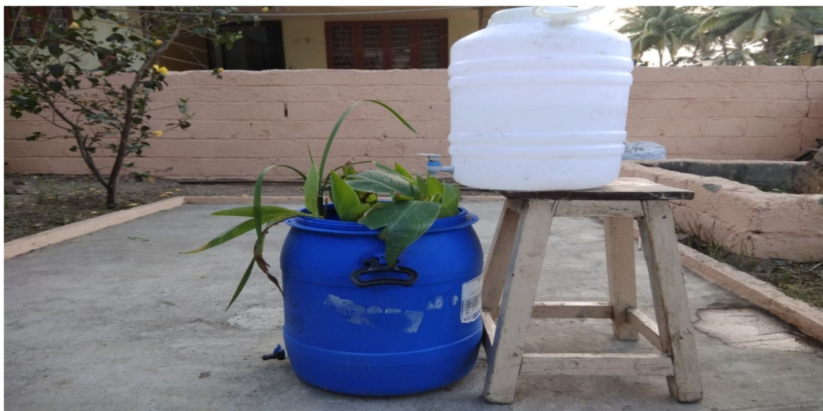
Fig.6.The Constructed Wetland used for pilot model.
