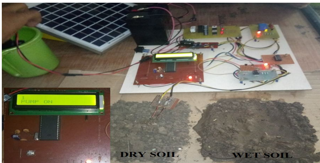
Fig. 6 Hardware Circuit of proposed system (Sensor is in DRY soil)
