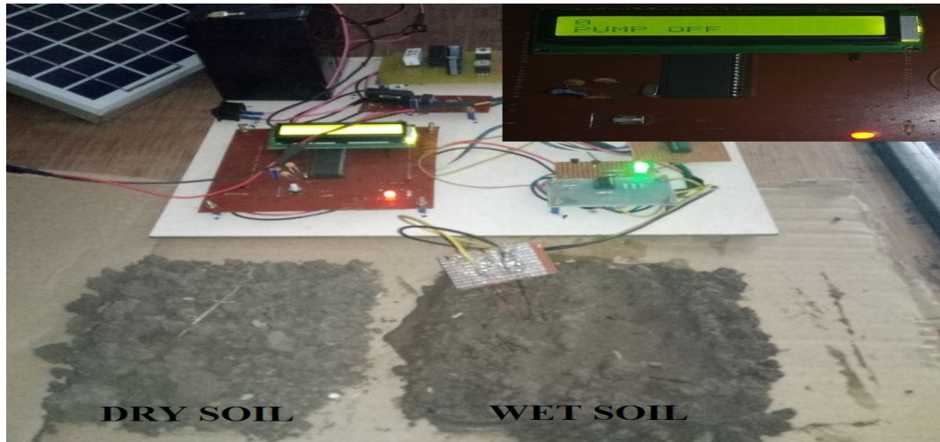
Fig. 7 Hardware Circuit of proposed system(Sensor is in WET soil)
