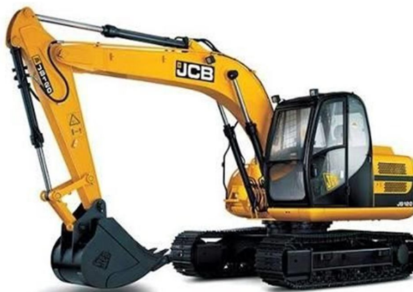
Fig-2: Excavator (Earthmoving machine)
