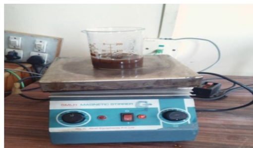
Fig 2: Synthesis of silver nanoparticles by reduction of \text{AgNO}_3 on magnetic stirrer.
