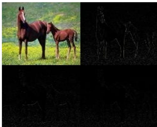
Fig6.1.2: Level 1 of 2D Haar wavelet decomposition
