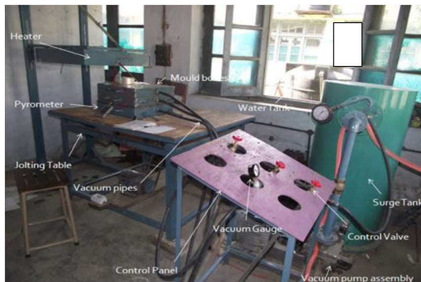
Fig. 2 The schematic view of vacuum moulding.
