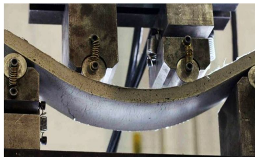
Testing of slab
