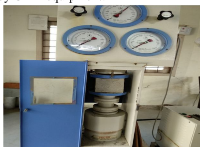
Compression test of a cube
