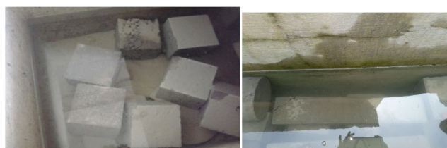
Curing of concrete cubes
