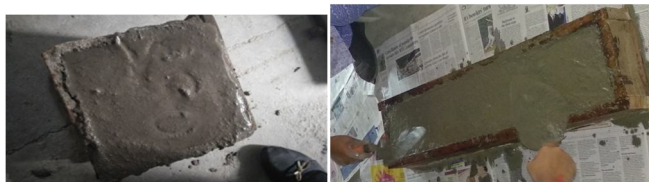
Casting of cube
