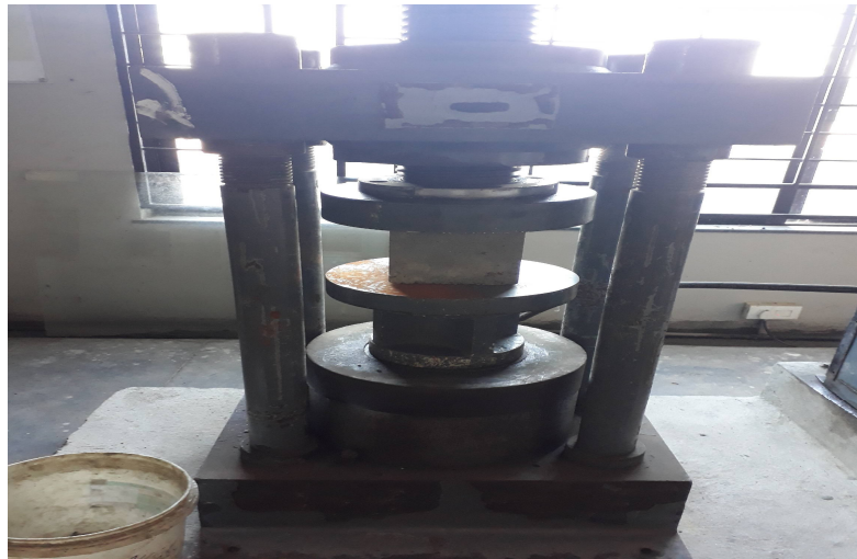
Fig: comp. Strength on cube specimen
