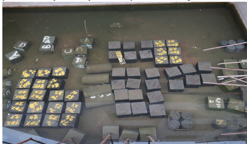
Fig: curing of cubes
