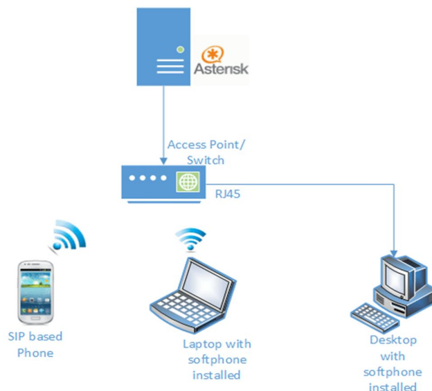
Fig. 1. Call between laptop, desktop and mobile phone on Wifi/ LAN through asterisk server.
