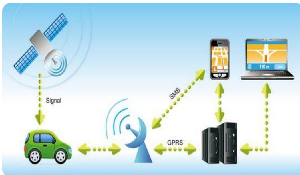
Fig. 1 Vehicle Tracking System Layout. Ref: http://currencyobserver.com
