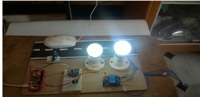
Figure 4 After detection of the vehicle the street lights are turned ON
