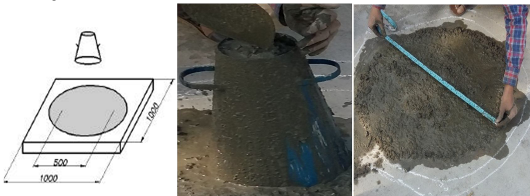
Figure 3: Slump Flow Test Equipment
