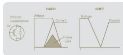
Fig-3. Hard and Soft Switching Waveform
